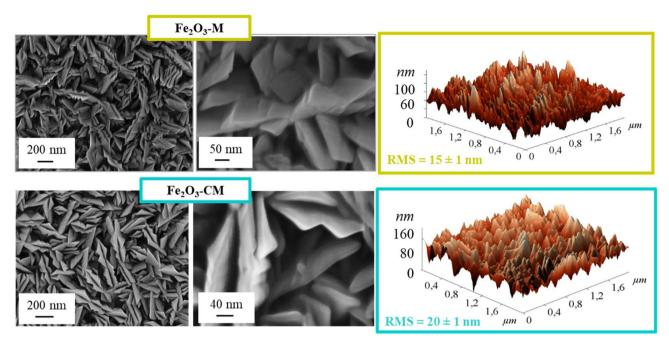
Fig. 1 Morphological characterization of  $Fe_2O_3$  deposits functionalized with gCN(M) (top panel) and gCN(CM) (bottom panel): FE-SEM (left) and AFM micrographs (right).
