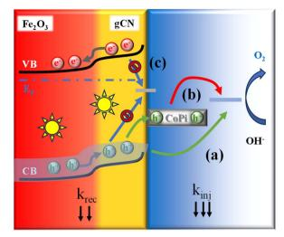
Fig. 9 Simplified model of the elementary processes taking place on the Fe<sub>2</sub>O<sub>3</sub>-gCN photoanode in the presence of CoPi. Photoexcited carriers move towards the semiconductor/electrolyte interface with direct water oxidation by VB holes (a), and charge transfer via a CoPi co-catalyst (b). Surface state-mediated recombination is appreciably depressed (c)
