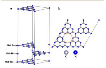
Fig. 12 (a) Schematic representation of three-layer g-C<sub>3</sub>N<sub>4</sub> model, (b)  $2 \times 2 \times 1$  supercell monolayer g-C<sub>3</sub>N<sub>4</sub>. The highlighted ring composed of six numbers of bi-coordinated nitrogen atoms is referred to as six-fold cavity. Reproduced with permission from ref. 7. Copyright 2018 Elsevier.
