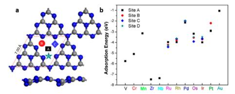
Fig. 27 (a) Possible adsorption sites for single metal atoms in  $g-C_3N_4$  layer, (b) adsorption energies of various metal single atoms on available adsorption sites in the  $g-C_3N_4$  surface. Reproduced with permission from ref. 115. Copyright 2020 American Chemical Society.
