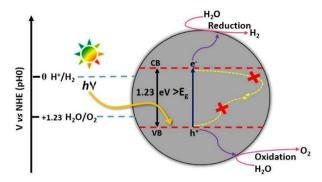
Fig. 15 Schematic diagram of photocatalytic water splitting.
