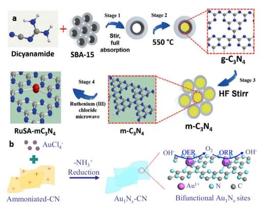
Fig. 7 (a) Schematic of microwave assisted post synthetic strategy for the development of ruthenium single atoms decorated mesoporous  $C_3N_4$  (RuSA- $mC_3N_4$ ) catalyst. Reproduced with permission from ref. 21. Copyright 2021 John Wiley and Sons. (b) Schematic of electrostatic adsorption mediated post synthetic strategy for  $Au_1N_x$  single-site/ $C_3N_4$  catalyst synthesis. Reproduced with permission from ref. 22. Copyright 2018 Elsevier.
