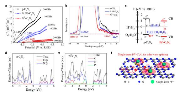
Fig. 18 (a) Mott–Schottky plot of  $Pt''-C_3N_4$  in comparison with  $g-C_3N_4$  and  $PtNP-C_3N_4$ , (b) UPS spectra of  $g-C_3N_4$ ,  $Pt''-C_3N_4$   $PtNP-C_3N_4$ , (c) schematic band structure alignment, DOS of (d)  $q-C_3N_4$  and (e)  $Pt''-C_3N_4$ , (f) mechanistic pathways (schematic) of the photocatalytic water splitting by Pt"-C<sub>3</sub>N<sub>4</sub> Reproduced with permission from ref. 23. Copyright 2018 American Chemical Society.
