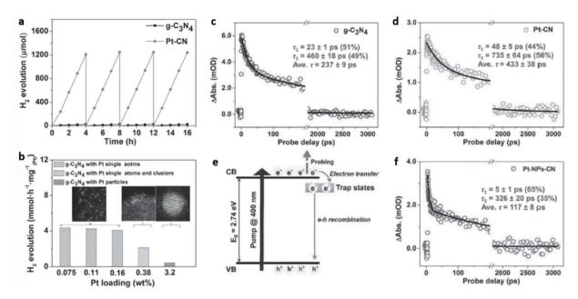
Fig. 16 (a) Photocatalytic  $H_2$  evolution with time for  $g-C_3N_4$  and Pt-CN, (b) photocatalytic  $H_2$  evolution with varying Pt content (normalised per Pt atom), average recovery life time values in mOD (optical density) of (c) g-C<sub>3</sub>N<sub>4</sub>, (d) Pt-CN, (e) an illustration of the various mechanisms involved, (f) data on TA kinetics for Pt-NPs-CN. Reproduced with permission from ref. 64. Copyright 2016 John Wiley and Sons.
