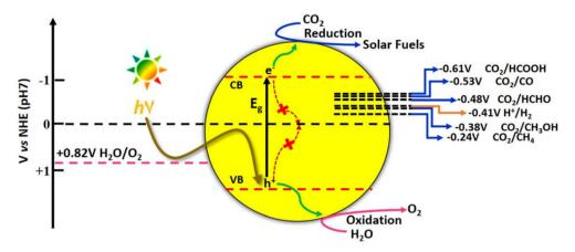
Fig. 13 Schematic illustration of photocatalytic carbon dioxide reduction.
