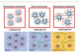
Fig. 2 Schematic diagram illustrating the three main mechanisms for particle stabilisation: steric and electrostatic interactions are represented with black lines and negative red charges respectively. Colloidal inks involve an electro-steric stabilization mechanism, which gives rise to polyelectrolyte complexes. The green lines represent the polymer chains within gel-embedded inks (reprinted with permission from ref. 60).
