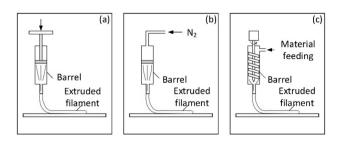
Fig. 3 Types of direct-writing extruders: (a) constant ram velocity; (b) constant pressure; (c) screw extrusion (adapted with permission from ref. 65).
