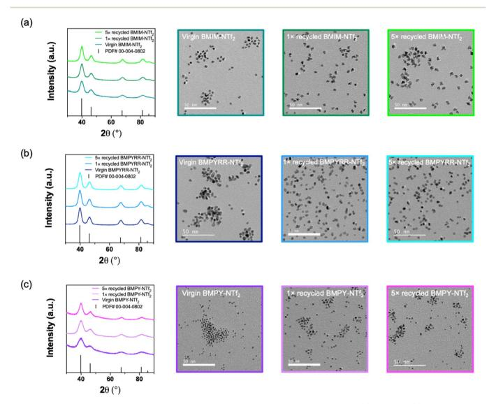
Fig. 3 Powder XRD patterns and TEM images of Pt nanoparticles synthesizing in virgin,  $1 \times$  and  $5 \times$  recycled (a) BMIM-NTf<sub>2</sub>, (b) BMPYRR-NTf<sub>2</sub>, and (c) BMPY-NTf<sub>2</sub>.
