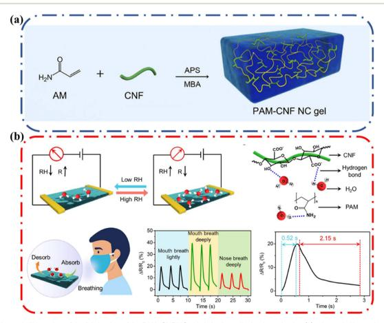
Fig. 17 (a) Schematic illustration of the fabrication of the PAM-CNF NC gel via in situ radical polymerization (b) schematic illustrating the humidity sensing mechanism of the CS-NC gel, the formation of hydrogen bonds between water and CNF, as well as water and PAM, schematic diagram of breath monitoring and resulting relative resistance changes of CS-NC sensors under different breath conditions. Reprinted with permission from Yu et al.77 Copyright 2022 American Chemical Society.
