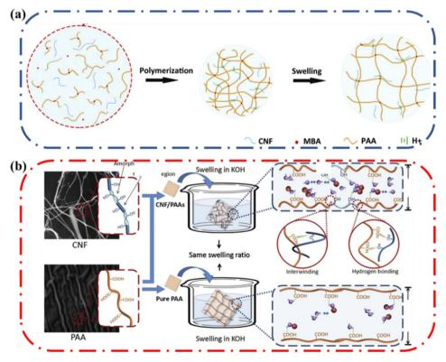
Fig. 7 (a) Schematic of polymerization and swelling of the cellulose nanofibrils (CNF)/poly(acrylic acid) (PAA) IC hydrogel (b) schematic picture of the mechanism of CNF/PAAs gel electrolyte and PAA electrolyte swelling in KOH in same swelling ratio. Reprinted with permission from Li *et al.*<sup>58</sup> Copyright 2018 Elsevier.
