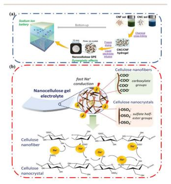
Fig. 10 (a) Schematic representation of the nanocellulose gel electrolyte fabrication. (b) Schematic illustration of the proposed Na<sup>+</sup> conduction mechanism across the nanocellulose Gel Polymer Electrolytes (GPE). Reprinted with permission from Mittal et al. 62 Copyright 2022 Wiley
