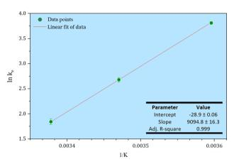
Fig. 10 A van't Hoff plot for estimation of the thermodynamic parameters of the arsenic adsorption process.
