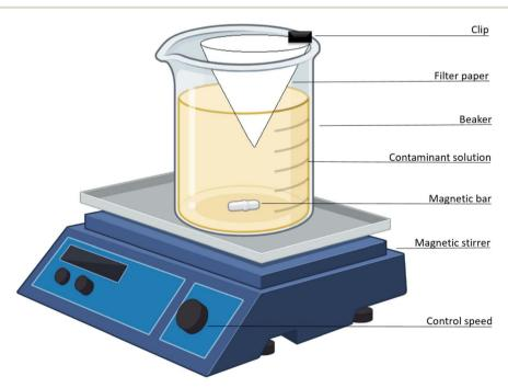
Fig. 1 Illustration of the one-pot method for in situ kinetic adsorption studies.
