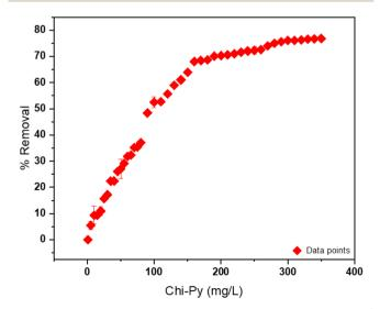
Fig. 7 Removal% and Chi-Py dosage evaluation from  $1-400~{\rm mg}~{\rm L}^{-1}$  with constant arsenic(v) concentration at 23 °C and pH 7.5.
