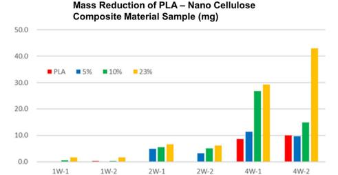
Fig. 4 Biodegradability test result. It can be seen that biodegradability increased as the content of nanocellulose increases in the PLA-nanocellulose composite material.<sup>49</sup>
