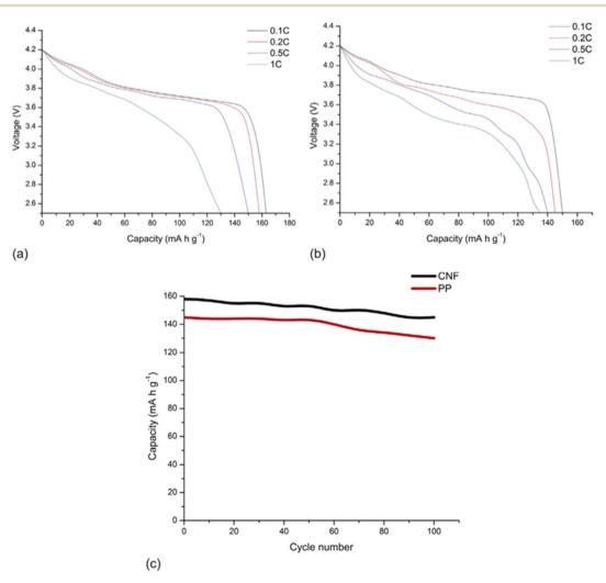
Fig. 14 Discharge profiles of cells with (a) CNF separator and (b) PP separator. (c) Comparison of cycling performance between CNF separator and PP separator. (c) Comparison of cycling performance between CNF separator.
