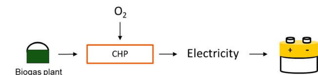
Fig. 1 Schematic representation of combined heat and power (CHP) production: independently from renewable energy availability, biogas is combusted to produce electricity.
