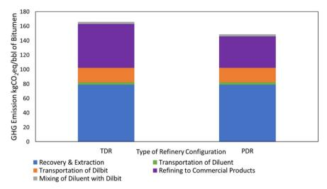
Fig. 11 WTT analysis on the deep configuration refinery. The GHG emission cycle for the TDR is 166 kg CO<sub>2eq</sub> per bbl of bitumen whereas for PDR it is 149 kg CO<sub>2eg</sub> per bbl of bitumen. This results in a GHG emission decrease of 10.3% when comparing the life cycle from WTT.
