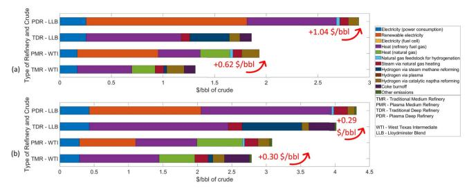
Fig. 7 (a) Comparison of energy cost with tax by using process units in different refinery scenarios. (b) Includes the carbon tax at a rate of \$0.05 per kg CO<sub>2eq</sub> from the GHG emissions in addition to the energy cost. Adding a carbon tax reduces the cost difference to 10%.
