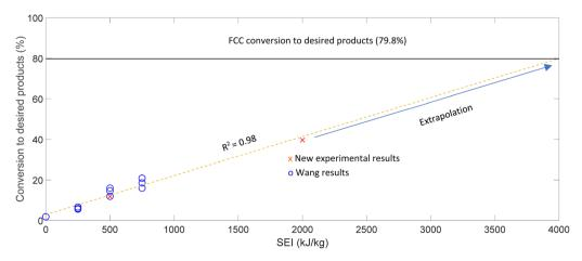
Fig. 1 SEI vs. overall conversion with new experimental results alongside Wang's prior results showing linear performance up to 2000 kJ kg $^{-1}$ and extrapolated to 4000 kJ kg $^{-1}$ . In an FCC, typically 79.8% of the feed is converted and the projected overall conversion for 4000 kJ kg $^{-1}$ similar to that of FCC.
