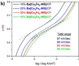
Fig. 5 (a) Rotating disk electrode linear sweep voltammetry (RDE-LSV) of  $Ba[Co_2Fe_2-WS]/CP$  electrodes at increasing catalyst loading in the CP blend. (b) Tafel plots obtained from the RDE-LSV data. The dashed lines indicate the Tafel regions. The experiments were conducted in a single-cell using a pH 7.2, 50 mM KP<sub>i</sub> buffer and KNO<sub>3</sub> (1 M) as electrolyte. The scan rate was 1 mV s<sup>-1</sup> at a rotation speed of 1600 rpm.
