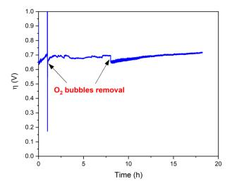
Fig. 6 Long-term stability of  $Ba[Co_2Fe_2-WS]/CP$  electrodes. Chronopotentiometry at 1 mA cm<sup>-2</sup> employing a 30 wt%  $Ba[Co_2Fe_2-WS]/CP$  electrode. The arrows indicate the removal of the  $O_2$  gas bubbles trapped on the electrode surface. The experiments were conducted in an H-cell using a pH 7.2, 50 mM KP<sub>i</sub> buffer and KNO<sub>3</sub> (1 M) as electrolyte.
