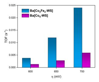
Fig. 9 Comparison of the calculated TOFs of Ba[Co<sub>2</sub>Fe<sub>2</sub>-WS] and Ba [Co<sub>4</sub>-WS] at different overpotentials during RDE-LSV measurements. The experiments were conducted using 30 wt% Ba[POM]/CP electrodes at pH = 7.2 using 50 mM KP<sub>i</sub> buffer and KNO<sub>3</sub> (1 M) as aqueous electrolyte. The scan rate was  $1 \text{ mV s}^{-1}$  and the rotational speed was 1600 rpm.
