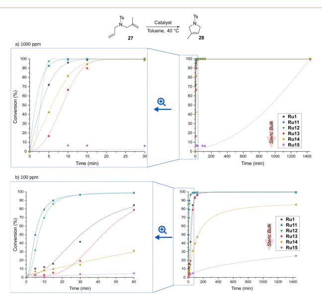
Scheme 7 Time/conversion curves for the RCM reaction of 2-allyl-2-(methylallyl)tosylate (27, 96% pure) with (a) 1000 and (b) 100 ppm of CAAC-based complexes (monitored by GC). Lines are visual aids only.
