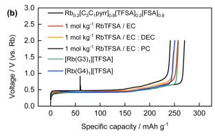
Fig. 5 (a) Galvanostatic reduction/oxidation curves of graphite electrodes in  $Rb_{0.2}[C_3C_1pyrr]_{0.8}[TFSA]_{0.2}[FSA]_{0.8}$  and  $Rb_{0.2}[C_3C_1pyrr]_{0.8}[TFSA]_{0.0}$  electrolyte. (b) Galvanostatic oxidation curves of graphite electrodes in non-aqueous organic electrolytes.
