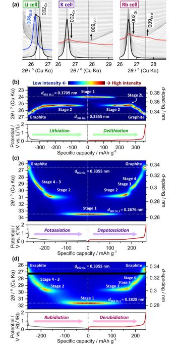
Fig. 4 (a) Operando XRD patterns of graphite electrodes during initial reduction processes in Li, K, and Rb cells. Operando XRD patterns as heat maps and corresponding reduction/oxidation curves of graphite electrodes during 2nd cycle in (b) Li, (c) K, and (d) Rb cells. The black line in the heat map of (d) is the area where diffraction caused by irregular orientation of a cell component was observed (see Fig. S9†).
