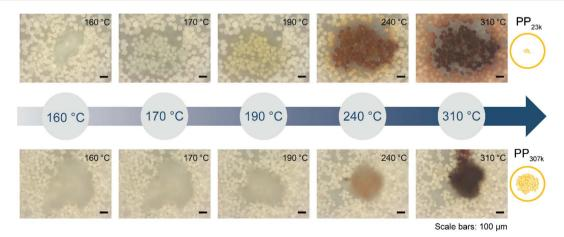
Fig. 6 In situ optical microscopy of polypropylene (PP) cracking using FCC catalyst. Individual polymer grains were placed on a bed of FCC catalyst and heated at 10 °C  $\min^{-1}$  under  $N_2$  flow in a Linkam stage. Images were acquired every minute. See ESI† for videos of the full reaction. Top: PP<sub>23k</sub>. Bottom: PP<sub>307k</sub>
