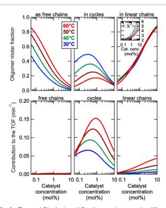
Fig. 5 (Top row) Distribution of O<sub>a</sub> oligomers between the different co-existing species in the  $O_a/O_{bi}$  systems (i = 1 or 2), depending on temperature and concentration, computed from the model. The inset in the right graph is the average degree of poly(oligomerization) by number of the linear chains vs. catalyst concentration. (Bottom row) Contribution of the different co-existing species to the catalytic turnover frequency, in the complete O<sub>a</sub>/O<sub>b1</sub> system.
