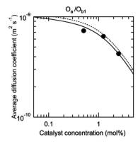
Fig. 4 DOSY-measured average diffusion coefficient of the protons of the oligomers in the complete O<sub>a</sub>/O<sub>b1</sub> system, depending on the concentration in M units (circles). The standard error is smaller than the point size. The curves are predictions based on the parameters from the fit of the catalytic activity, assuming either good (continuous curve) or  $\Theta$  (dotted curve) solvent conditions (ESI Section 9†).
