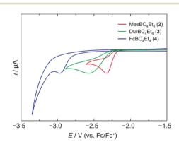
Fig. 2 Cyclic voltammograms of 2, 3, and 4 in dichloromethane solution showing the first reduction events (supporting electrolyte:  $[NBu_4][PF_6]$  (0.1 M), scan rate: 250 mV s<sup>-1</sup>).
