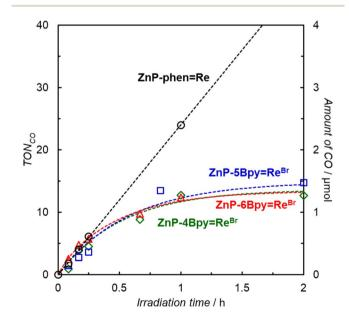
Fig. 7 Time dependence of CO formation (0-2 h) during irradiation at 420 nm by LED lamps (input power: 30 mW), in a merry-go-round irradiation apparatus, of CO2-saturated DMA solutions containing the dyad (0.05 mM) and BIH (0.05 M).
