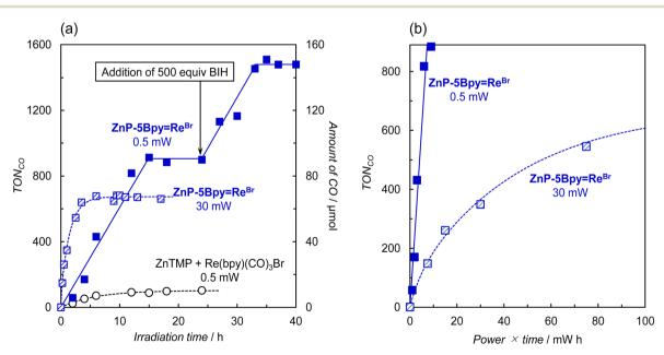
Fig. 10 (a) Time dependence of CO formation during irradiation at 420 nm by LED lamps (input power: 0.5 and 30 mW), in a merry-go-round irradiation apparatus, of  $CO_2$ -saturated DMA-TEOA (4:1 v/v) solutions containing ZnP-5Bpy=Re<sup>Br</sup> (0.05 mM), and a mixed system of ZnTMP (0.05 mM) and fac-Re(bpy)(CO)<sub>3</sub>Br (0.05 mM) in the presence of BIH (0.05 M). (b) Plots of  $TON_{CO}$  versus product of input power and irradiation time.
