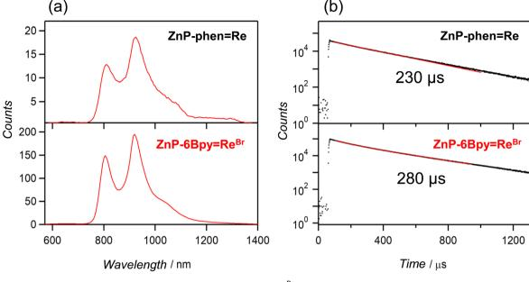
Fig. 5 (a) Phosphorescence spectra of ZnP-phen—Re and ZnP-6Bpy—Re<sup>Br</sup> in Ar-saturated DMA ( $\lambda_{ex} = 405$  nm) at room temperature. The spectra were recorded with delay time > 90 μs after the excitation pulse. (b) Phosphorescence decay profiles (semilog plot) of ZnP-phen—Re and ZnP-6Bpy=Re<sup>Br</sup> in Ar-saturated DMA ( $\lambda_{ex} = 405$  nm) at room temperature, monitored at 800 and 920 nm. The decay profiles were fitted with one component (red lines).
