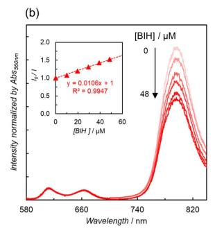
Fig. 6 (a) Comparison of emission spectra of ZnP-nBpy=Re<sup>Br</sup> in Ar-saturated DMA ( $\lambda_{ex} = 560$  nm) at 298 K. (b) Emission spectra of ZnP-6Bpy=  $Re^{Br}$  in the presence of various amounts of BIH in Ar-saturated DMA ( $\lambda_{ex} = 560$  nm) at 298 K. Inset shows Stern-Volmer plot of the emission.
