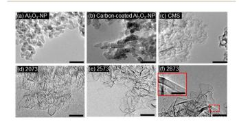
Fig. 2 TEM images of (a)  $Al_2O_3$ , (b) carbon-coated  $Al_2O_3$ , (c) CMS, and annealed samples at (d) 2073 K, (e) 2573 K, and (f) 2873 K. The scale bar is 20 nm. The highly stacked graphene structure in (f) was highlighted and magnified (the scale bar in magnified part is 10 nm).
