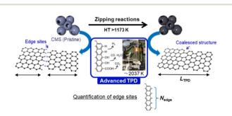
Fig. 1 Schematic of HT of CMS and the acommpanied graphene-zipping reactions. The advanced temperature-programmed desorption (TPD) is used to quantify the carbon edge sites and calculate the average graphene-domain size  $(L_{\text{TPD}})$ .
