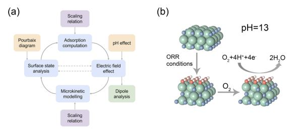
Fig. 5 (a) An illustration of the proposed analytical framework. (b) The alkaline ORR mechanism on ZrN. Green, blue, red, and white spheres denote Zr, N, O, and H, respectively.
