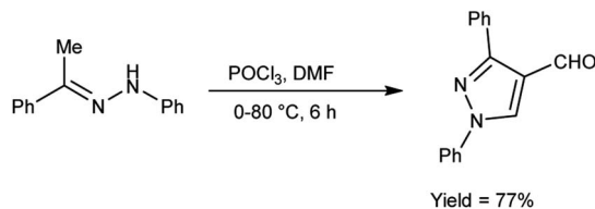
Scheme 19 Synthesis of 1,3-diphenylpyrazole-4-carboxaldehyde.
