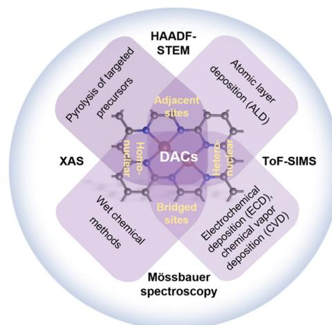
**Fig. 2** Illustration of the preparation and characterization methods of DACs. HAADF-STEM: high-angle annular dark-field scanning transmission electron microscopy; XAS: X-ray absorption spectroscopy; ToF-SIMS: time-of-flight secondary ion mass spectrometry.
