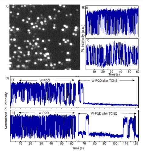
Fig. 3 PET-induced blinking of single-PQDs. (A) A PL image of W-PQDs on a cover glass substrate and photoexcited at 404 nm (585 W cm<sup>-2</sup>). (B) PL intensity trajectories of two pristine W-PQDs. (C) Real-time PL intensity trajectories of single W-PQD immersed in 1-hexadecene (from 0 to 62 s) before and (from 65 to 120 s) after the addition of (i) TCNB (1 mM in toluene) or (ii) TCNQ (1 mM in toluene). The bin size is 33 ms.
