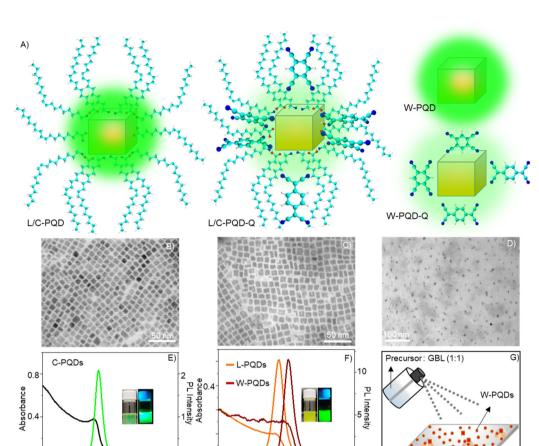
Fig. 1 Structures and optical properties of PQDs. (A) Schemes of PQDs with or without electron acceptors (quenchers, Q = TCNQ/TCNB). (B–D) TEM images of (B) C-PQDs, (C) L-PQDs, and (D) W-PQDs. Absorption and PL spectra of (E) C-PQDs and (F) L-PQDs and W-PQDs (insets: photographs of C/L-PQD solutions taken under room or UV light). The PL spectra were recorded under 400 nm excitation. (G) A scheme of the spray synthesis method.
