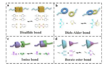
Fig. 1 The schematic diagram of reversible reaction of disulfide bonds (a), DA bonds (b), imine bonds, (c) and boronic ester bonds (d).
