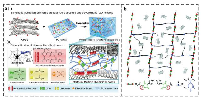
Fig. 7 (a) (i) Schematic of the PU-graphene oxide network with an inverse artificial nacre structure. (ii) Dynamic bond interaction in the biomimetic composite.<sup>2</sup> (b) The structure of cross-linked networks of RCFA.<sup>6</sup>
