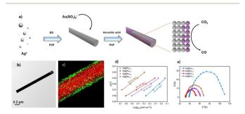
Fig. 4 (a) Schematic preparation process of Ag@Au core-shell nanowires. (b) Representative TEM image. (c) HAADF-STEM elemental mapping. (d) Tafel slope of Ag@Au<sub>0.2</sub>, Ag@Au<sub>0.5</sub>, Ag@Au<sub>0.8</sub> and Ag@Au<sub>1</sub> electrocatalysts. (e) EIS characterization of Ag@Au<sub>0.2</sub>, Ag@Au<sub>0.5</sub>, Ag@Au<sub>0.8</sub> and Ag@Au<sub>1</sub>
