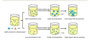
Fig. 2 Effect of the different concentrations of silver nitrate on the silver nanowire diameter. Reproduced with permission from ref. 38. Copyright 2019, MDPI.
