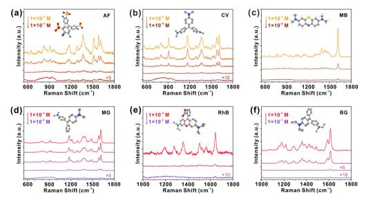
Fig. 4 Raman spectra of the detected chemicals by using 2D Mo<sub>4/3</sub>B<sub>2</sub> MBene SERS substrates. Raman spectra of (a) AF, (b) CV, (c) MB, (d) MG, (e) RhB, and (f) BG molecules with different concentrations adsorbed on the 2D Mo<sub>4/3</sub>B<sub>2</sub> MBene substrates.
