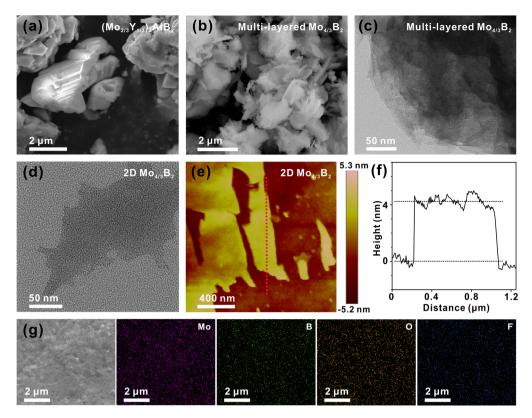
Fig. 2 Characterizations of the surface morphologies of MAB, multi-layered, and 2D  $Mo_{4/3}B_2$  MBenes. (a and b) SEM images of  $(Mo_{2/3}Y_{1/3})_2AlB_2$  and multi-layered  $Mo_{4/3}B_2$  MBene. (c and d) TEM images of multi-layered and 2D  $Mo_{4/3}B_2$  MBenes. (e) AFM image of 2D  $Mo_{4/3}B_2$  MBene. (f) Line profile across the dashed line in the image (e). (g) SEM image and the corresponding elemental mapping images of the 2D  $Mo_{4/3}B_2$  MBene substrate.
