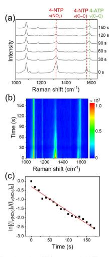
Fig. 3 (a) Time-dependent SERS spectra of 4-NTP and (b) corresponding color-coded intensity map of the SERS spectra obtained after the treatment of an aqueous solution of NaBH $_4$  onto the device. (c) Plot of the logarithm of the intensity of  $\nu(NO_2)$  peak relative to that of the initial stage *versus* the reaction time.
