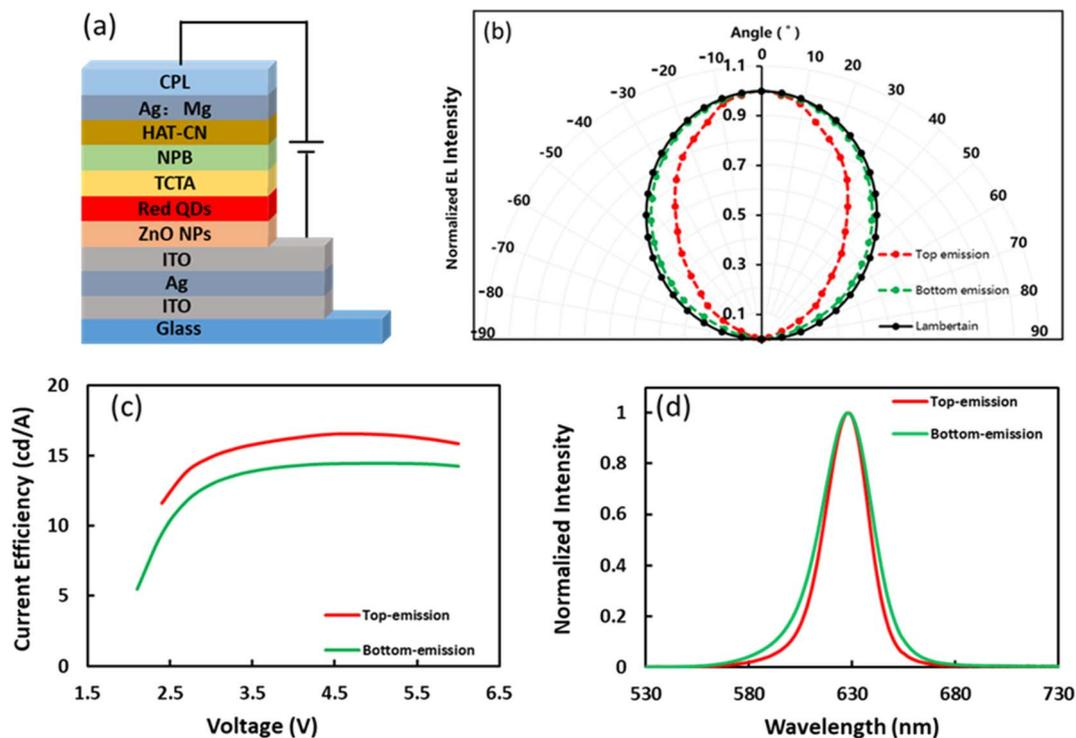
Fig. 4 (a) Schematic device architecture of PM top-emission QLED devices, (b) normalized angular-dependent EL intensity, (c) current efficiency curves and (d) comparison of the normalized electroluminescent spectra of the bottom and top emission QLEDs.
