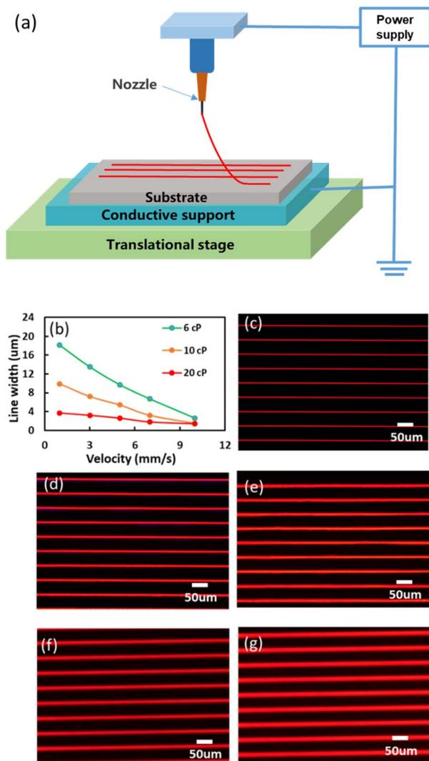
Fig. 1 (a) Schematic illustration of the EHD printing system comprising a single nozzle, a movable platform, a conductive platform and a power supply system, (b) and (c–g) fluorescence images of patterned lines with QD ink of 6 cP at printing speeds of  $10 \text{ mm s}^{-1}$ ,  $7 \text{ mm s}^{-1}$ ,  $5 \text{ mm s}^{-1}$ ,  $3 \text{ mm s}^{-1}$  and  $1 \text{ mm s}^{-1}$ , respectively.
