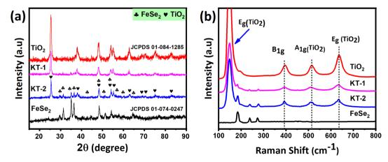
Fig. 1 (a) Crystal structure and (b) vibrational modes of the FeSe<sub>2</sub>, TiO<sub>2</sub>, KT-1, and KT-2 composite.
