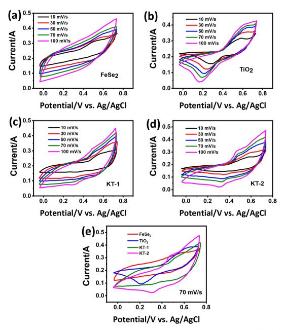
Fig. 5 Energy storage characteristics of the samples in a three-electrode setup for the electrode materials, CV curves of (a) FeSe<sub>2.</sub> (b) TiO<sub>2.</sub> (c) KT-1, (d) KT-2, and (e) comparative CV curves for all electrodes.
