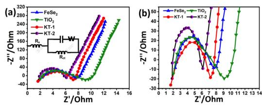
Fig. 7 (a) Impedance plots, inset is the equivalent circuit model, and the (b) zoomed view.
