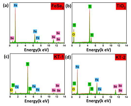
Fig. 3 EDX of (a) FeSe<sub>2</sub> and (b) TiO<sub>2</sub>, and (c) KT-1 (d) KT-2 composites.
