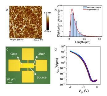
Fig. 5 Characterizations of the FETs fabricated by SWCNTs synthesized from coal. (a) AFM image of the SWCNT membrane on the Si substrate, size: 1 µm. (b) Length distribution of the SWCNTs sorted by PCz. (c) Optical photograph of the FET, objective:  $50\times$ . (d) Transfer characteristic curves of 10 FETs fabricated by the semiconducting SWCNTs sorted by PCz.
