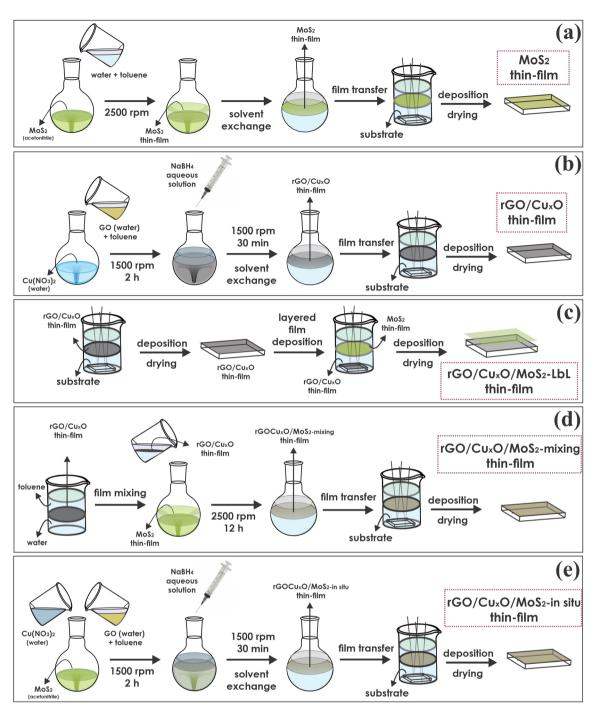
Fig. 1 Schematic representation of the general steps for the thin film preparation: (a) MoS<sub>2</sub>; (b) rGO/Cu<sub>x</sub>O or rGO; (c) rGO/MoS<sub>2</sub>-LbL and rGO/Cu<sub>x</sub>O/ MoS<sub>2</sub>-LbL; (d) rGO/MoS<sub>2</sub>-mixing and rGO/Cu<sub>x</sub>O/MoS<sub>2</sub>-mixing; (e) rGO/MoS<sub>2</sub>-in situ and rGO/Cu<sub>x</sub>O/MoS<sub>2</sub>-in situ
