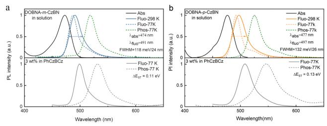
Fig. 2 UV-vis absorption and photoluminescence spectra of (a) DOBNA-m-CzBN and (b) DOBNA-p-CzBN in diluted toluene (upper) and in PhCzBCz films (below).
