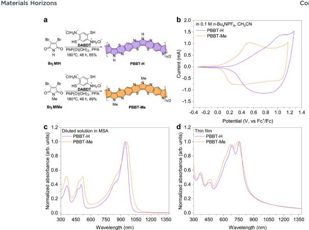
Fig. 1 Synthesis and physicochemical properties of PBBT-H and PBBT-Me. (a) Synthetic route of PBBT-H and PBBT-Me. (b) CV of PBBT-H and PBBT-Me. in 0.1 M n-Bu<sub>4</sub>NPF<sub>6</sub> acetonitrile solution. (c) and (d) UV-vis-NIR absorption spectra of PBBT-H and PBBT-Me in diluted MSA solutions (c) and thin films (d).
