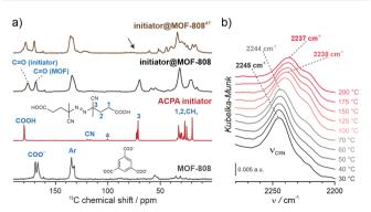
Fig. 2 Thermal decomposition of the ACPA initiator. (A)  $^{13}$ C CP-MAS spectra of MOF-808, pristine ACPA, and <code>initiator@MOF-808</code> before and after thermal activation; the arrow indicates a signal sensitive to the initiator thermal activation. (B) VT-DRIFT spectra of <code>initiator@MOF-808</code> (the C $\equiv$ N vibration range) measured in the temperature range of  $^{3}$ O-200  $^{\circ}$ C.
