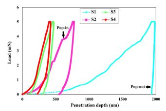
The load-displacement curves of the electrodeposited specimens.
