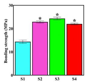
Coating-substrate adhesion strength values (\*p < 0.0001 vs. S1).
