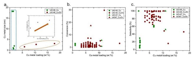
Fig. 14 (a) Cu metal size *versus* Cu metal loading (b) conversion of CO<sub>2</sub> *versus* Cu metal loading (b) selectivity towards methanol *versus* Cu metal loading.
