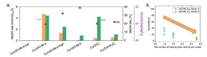
Fig. 11 (a) Rates of methanol (MeOH) production (orange bars), methanol selectivity (green bars) on selected catalysts at 250 °C and 32 bar, and activation energy ( $E_a$ , pink points). Reproduced from ref. 43 (https://www.nature.com/articles/s41467-020-19438-w) with the permission of unrestricted use (https://creativecommons.org/licenses/by/4.0/). (b) Selectivity toward methanol *versus* the number of missing linker defects per cluster.<sup>40,43</sup>
