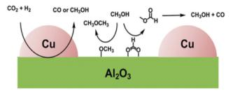
**Fig. 4** CO<sub>2</sub> hydrogenation on Cu/Al<sub>2</sub>O<sub>3</sub>. Used with permission of Angewandte Chemie International Edition, from CO<sub>2</sub> Hydrogenation on Cu/Al<sub>2</sub>O<sub>3</sub>: role of the metal/support interface in driving activity and selectivity of a Bifunctional Catalyst, Lam *et al.*, 2019, **58**, 39 permission conveyed through Copyright Clearance Center, Inc.
