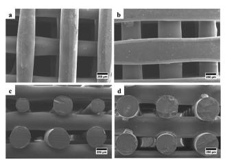
Fig. 4 SEM images of the fabricated scaffolds that were taken from the top-view: (a) PCL and (b) PCL/AgNPs; and the side-view: (c) PCL and (d) PCL/AgNPs.
