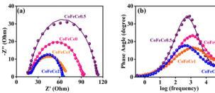
Fig. 8 (a) Nyquist plots, and (b) Bode plots at a bias potential of 1.54 V vs. RHE in the frequency range from  $10^5$  to  $10^{-1}$  s<sup>-1</sup> with 0.005 V amplitude for different LDHs. The experimental results are represented by discrete points and equivalent circuit fitted results are represented by solid lines.
