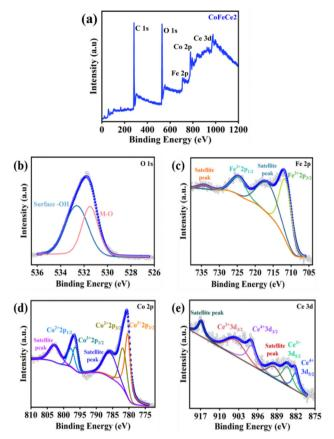
Fig. 3 XPS spectra of CoFeCe2. (a) XPS survey scan, (b) deconvoluted O1s spectra, (c) deconvoluted Fe2p spectra, (d) deconvoluted Co2p spectra, and (e) deconvoluted Ce3d spectra.
