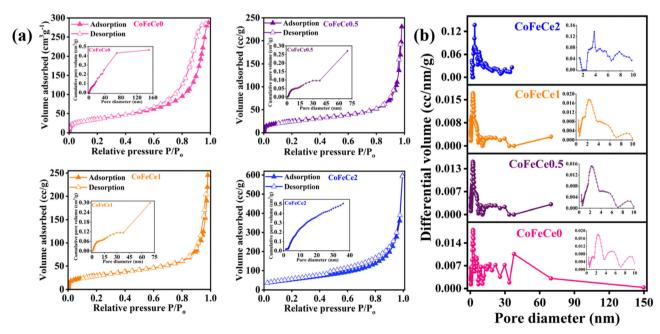
Fig. 4 (a) N<sub>2</sub> adsorption-desorption isotherm profile at 77 K. Insets show the cumulative pore volume of the respective samples, and (b) pore size distribution (inset shows small pore region) of Ce-doped CoFe LDHs.
