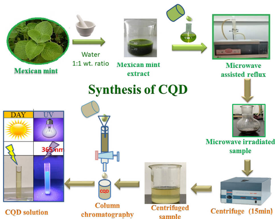
Fig. 4 Synthesis process of CQDs by microwave method reproduced with permission from ref. 29 Copyright © 2021 Elsevier.
