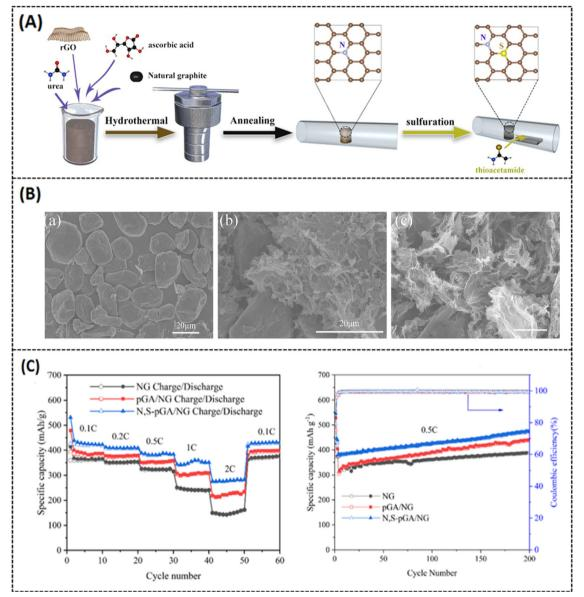
Fig. 4 (A) Schematic representation of N, S-PGA/NG, (B) (a-c) SEM images of pure graphene, PGA/NG and optimal N, S-PGA/NG, (C) rate performance at different current densities and cycling performance at 0.5C current density. Reprinted with permission, <sup>41</sup> Copyright (2021) from Elsevier.
