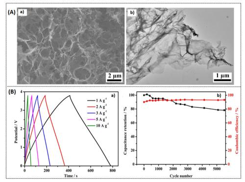
Fig. 13 (A) SEM images of (a) UPGA and (b) TEM image of UPGA, (B) electrochemical Response of UPGA: (a) GCD response (b) cycling stability vs. coulombic efficiency at 1 A g<sup>-1</sup>. Reprinted with permission, <sup>93</sup> Copyright (2021) from Elsevier.
