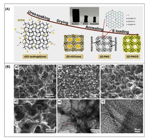
Fig. 6 (A) Schematic illustration of the preparation process of 3D-PNG/S composites, (B) (a and b) SEM images of 3D-FGO, 3D-FGO@ures, (c and d) low-high-magnification of 3D-PNG (e and f) TEM image of 3D-PNG, HRTEM image of the marked area in. Reprinted with permission, <sup>56</sup> Copyright (2019) from Flsevier
