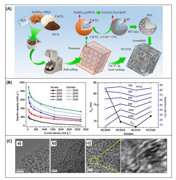
Fig. 3 (A) Schematic representation of porous carbon network, (B) capacitance at different current densities from 50 to 3200 mA g<sup>-1</sup>, (d) comparative response of retention rate vs. D average of different samples at various current densities, (C) TEM images of the optimal sample at different magnifications. Reprinted with permission, <sup>40</sup> Copyright (2021) from Elsevier.
