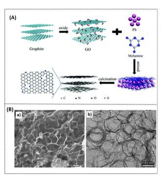
**Fig. 10** (A) Schematic representation of preparation protocol of N-3DPG, (B) (a and b) FE-SEM and TEM images of N-3DPG. Reproduced with permission, <sup>72</sup> Copyright (2017), Royal Society of Chemistry.
