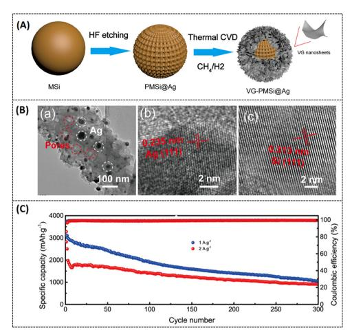
Fig. 5 (A) Schematic representation of the as-prepared VG-PMS@Ag, (B) (a-c) TEM images of the PMS@Ag composite, interplanar spacing of Ag in PMS@Ag, interplanar spacing of Silicon in PMS@Ag. (C) Long-term cycling activity of the VG-PMS@Ag electrode at different applied current densities. Reprinted with permission, <sup>42</sup> Copyright [2022] American Chemical Society.
