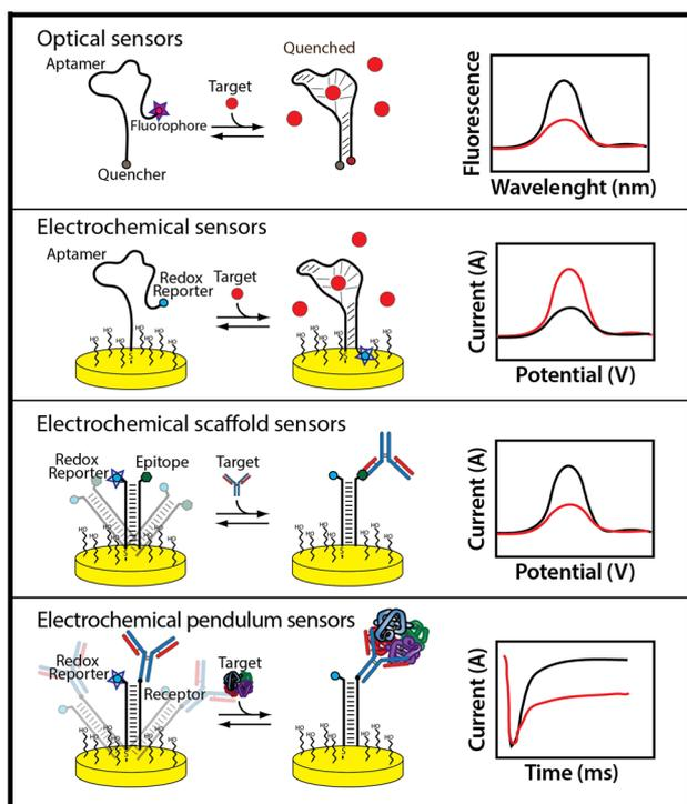
**Fig. 4** Employing binding-induced conformational change to produce an optical or electrochemical output appears an excellent option for performing continuous, real-time molecular monitoring in support of feedback control functionalities.
