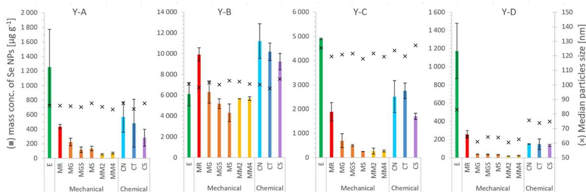
Fig. 4 SeNP mass per g of selenized yeast, and the median size, after the extraction procedure: E—enzymatic,<sup>16</sup> MR—mechanical,<sup>20</sup> MG—glass beads, MGS—glass beads and sand, MS—sand, MM2—2 metal beads, MM4—4 metal beads, CN—1000 mM NaOH, CT—4% TMAH, and CS—4% SDS. Each column and error bar represent average and SD of two replicates, respectively.
