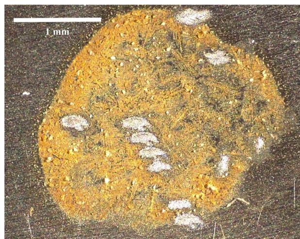
Fig. 2 Optical micrograph of sample BCR-2B deposited on a Ti metal substrate. The desorption laser spots from multiple analyses are clearly visible.
