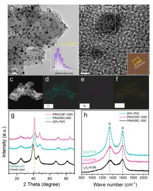
Fig. 2 (a) HRTEM image and particle size distribution (inset) for PtNi/ CNF-1200; (b) HRTEM image for PtNi/CNF-1200, the inset shows the corresponding information about lattice fringes; (c) HRTEM image and (d-f) energy-dispersive X-ray spectroscopy (EDS) mapping for PtNi/ CNF-1200; (g) XRD patterns and (h) Raman spectra for PtNi/CNF-1200, PtNi/KBC-600, and 20% Pt/C.
