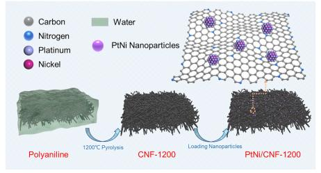
Fig. 1 Schematic illustration of the fabrication of PtNi/CNF-1200
