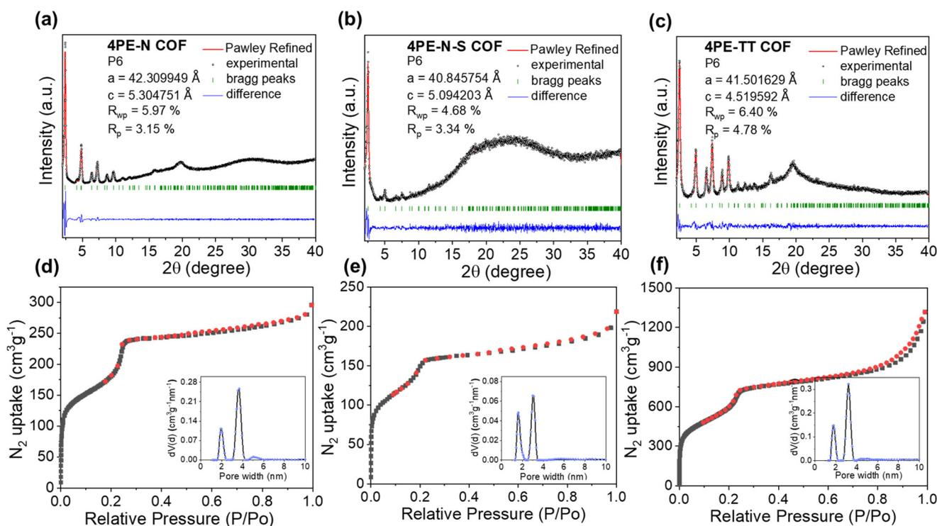
Fig. 2 The PXRD patterns and Pawley refinements of (a) 4PE-N-COF, (b) 4PE-N-S-COF and (c) 4PE-TT-COF.  $\text{N}_2$  adsorption/desorption isotherms and pore size distributions (inset) of (d) 4PE-N-COF, (e) 4PE-N-S-COF and (f) 4PE-TT-COF.
