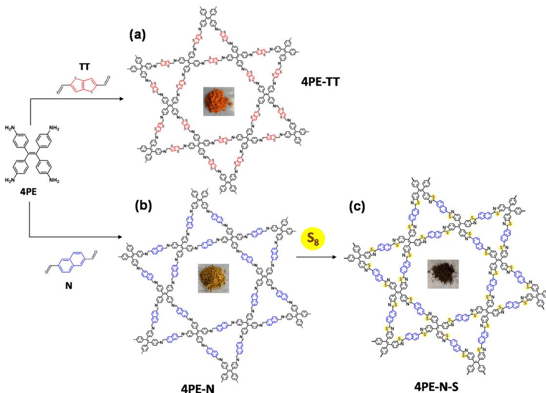
Fig. 1 Schematic for the synthesis of (a) 4PE-TT, (b) 4PE-N, and (c) 4PE-N-S COFs.
