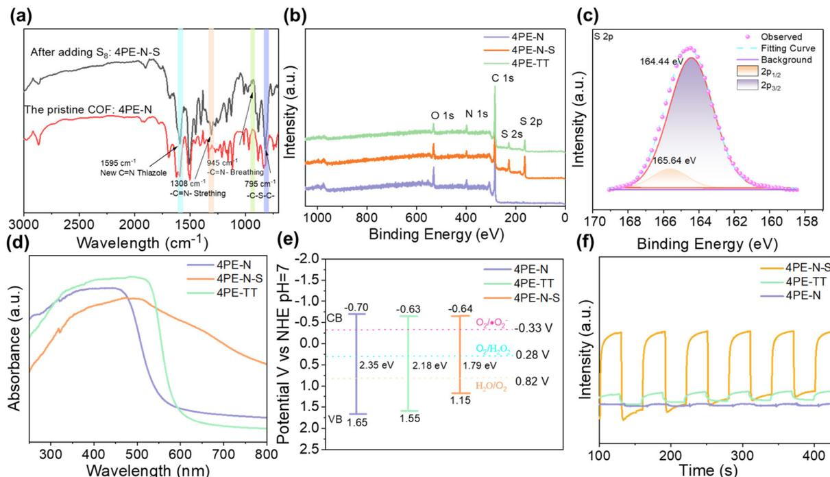
**Fig. 3** (a) FT-IR spectrum of 4PE-N and 4PE-N-S COFs, (b) survey XPS spectrum of all samples in the region of C 1s, N 1s, O 1s, and S 2p, (c) XPS spectra of 4PE-N-S in the region of S 2p, (d) UV-vis spectra, (e) band alignment and (f) photocurrent responses of 4PE-N, 4PE-N-S and 4PE-TT COFs.
