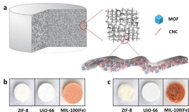
**Fig. 6** a) Schematic of MOF-cellulose hybrid aerogel, b) photographs of CNC-CMC based hybrid aerogels (CNC:CMC:MOF = 1:1:1 by weight), and c) all-CNC based hybrid aerogels (CNC:CNC:MOF = 1:1:1 by weight); aerogels are about 7 mm in diameter and 5 mm in height (reproduced from ref. 125 with permission from Wiley, copyright 2016).
