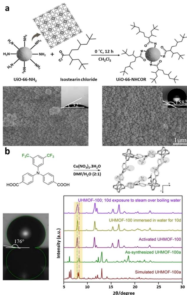
**Fig. 3** (a) Post-synthetic modification of UiO-66-NH<sub>2</sub> with isostearin chloride to reduce hydrophilicity (reproduced from ref. 88 with permission from Elsevier Inc., copyright 2019). (b) Synthesis of UHMOF-100, with the use of trifluoromethyl groups on the ligand to generate an ultra hydrophobic MOF (reproduced from ref. 89 with permission from Wiley, copyright 2016).
