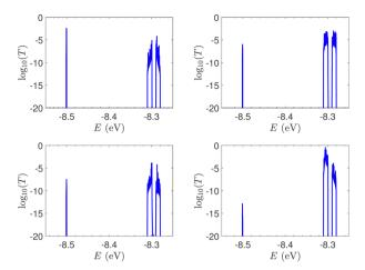
Fig. 11 The  $log_{10}(T(E))$  of the studied sequences (ideal geometries) with STR expansion mutations. Upper left: Huntington's disease with 100 STR expansions, upper right: Kennedy's disease with 45 STR expansions, left lower: Spinocerebellar ataxia 6 with 30 STR expansions, lower right: Spinocerebellar ataxia 7 with 100 STR expansions.
