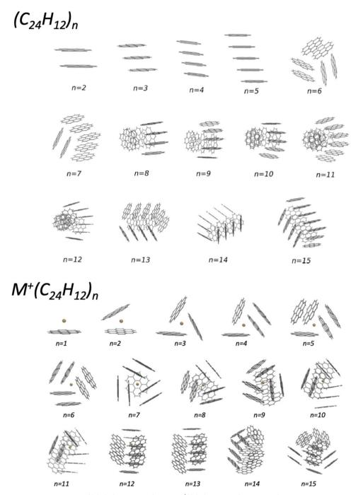
Fig. 2 Putative global minimum structures of (COR)<sub>n</sub> (upper panel) and of K<sup>+</sup>(COR)<sub>n</sub> clusters (lower panel) with n = 1-15. They have been obtained by exploiting a detailed global optimization study with an evolutionary algorithm (see the text). 51,53
