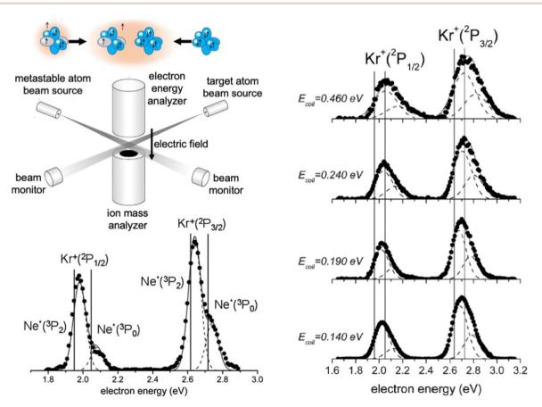
Fig. 7 A schematic view of the experimental apparatus used in the Perugia laboratory to measure the collision energy (Ecoil) dependence of partial, total ionization cross sections and PIES. Plotted PIES refer to Ne\* $(^{3}P_{J})$  + Kr entrance channels leading to the formation of Ne + Kr $^{+}(^{2}P_{J})$  ionic products.
