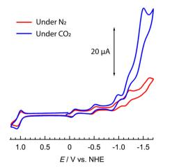
Fig. 2 Cyclic voltammetry of  $\bf 1$  (1 mM) under  $N_2$  (red) or  $CO_2$  (Blue) in NMP, with 0.1 M  $^{n}\mathrm{Bu_{4}NPF_{6}}$  supporting electrolyte vs. NHE redox couple. Glassy carbon working electrode (d = 3 mm), Pt wire counter electrode, and a SCE reference (corrected to NHE, see ESI†).
