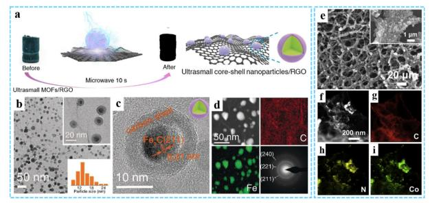
Fig. 8 (a) Schematic illustration of the fabrication process of  $Fe_3C@C/RGO$ . (b) TEM and (c) HRTEM images of  $Fe_3C@C/RGO$ . (d) STEM image, element mapping and SAED pattern. Reproduced with permission from ref. 78 Copyright 2020 Wiley-VCH. (e) SEM image of CoN<sub>x</sub>/NGA. (f) HAADF and (g)-(i) EDXS images of CoN<sub>x</sub>/NGA. Reprinted with permission from ref. 52. Copyright 2019 Elsevier.
