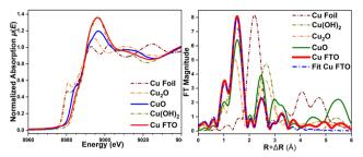
Fig. 5 (a) Normalized XANES spectra  $\mu(E)$  and (b) Fourier-Transform  $FT|k^3\gamma(k)|$  spectra of the Cu deposit and reference oxides, and fitting to
