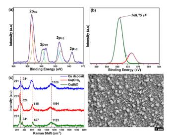
Fig. 4 XP spectrum of the Cu deposit on FTO (after CPE) showing (a) Cu 2p and (b) Cu LMM regions. (c) Raman spectra of the Cu deposit, CuO and Cu(OH)<sub>2</sub>. (d) SEM image of the FTO electrode after 7 h of CPE.
