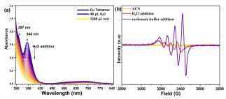
Fig. 1 (a) In situ UV-Vis spectra of the Cu-tetramer upon serial addition of water. (b) X-band EPR spectra of the Cu-tetramer on adding water and 0.08 M carbonate buffer (pH 10.5).
