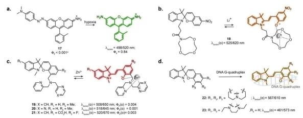
Fig. 5 Examples of conventional biosensors and reactive probes based on photoswitches. The properties reported were measured in: aqueous buffer at pH = 7.0 - 7.4 for 17, 19, 20, 22 and 23; aqueous buffer pH = 7.4 containing 50% MeCN for 18;  $H_2O$  for 21; The notation (o) refers to the open isomer, after binding or chelation.
